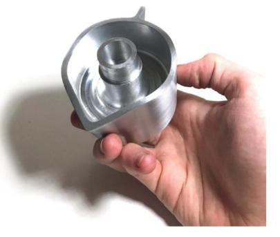
ensured that the two cuts would align perfectly, giving even wall thicknesses around the piece.
