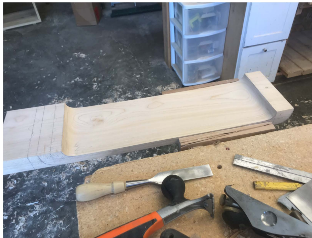
Continued roughing out
